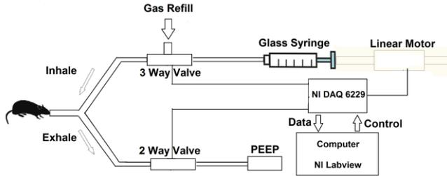
Fig. 1 Constructed mechanical ventilator's block diagram
