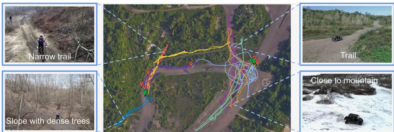
**FIGURE 19** Testing facility. The middle figure shows a top-down satellite view of testing terrain, overlaid with unmanned aerial vehicle positions from different trials. We accumulated over 2 hr of flight time and a total distance of almost 6 km. The side figures show the diverse types of terrains in our experiments. The figures also depict different actors and different seasons [Color figure can be viewed at [wileyonlinelibrary.com](http://wileyonlinelibrary.com)]
